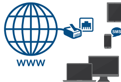
TAEvo Tech can be integrated with supervision system using the kit RS485 and the kit xWEB300D operating via Internet.
