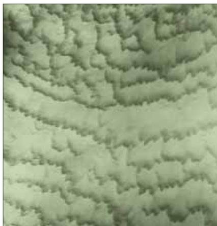
A high speed photo of the liquid distribution on the Centritherm Cone
